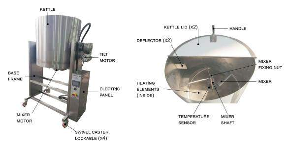
Figure 1: Structural components of the machine
