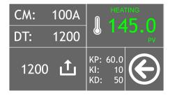
Figure 7: PID regulator screen
